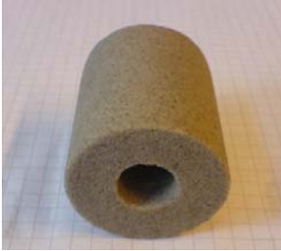
Figure 7. The Berea sandstone with drilled tube like cavity.
