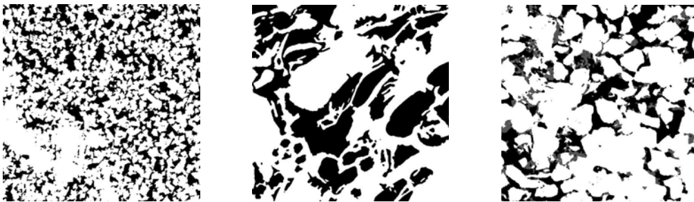
Figure 2. From left to right; cross-sectional images of the MCT samples C1, C2 and S1. The side lengths are 0.84 mm, 1.55 mm and 2.68 mm, respectively. In the images, black is the pore space; grey is clay; and white is the solid matrix.
