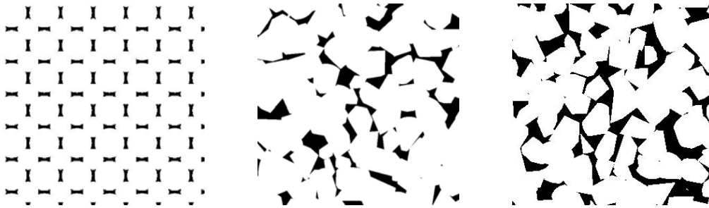
Figure 1. From left to right: cross-sectional images of sample P1, F11 and F22 generated using the PB method. The side lengths are 0.375 mm, 1.5 mm and 1.5 mm respectively. In the images, black is the pore space; white is the quartz grain.
