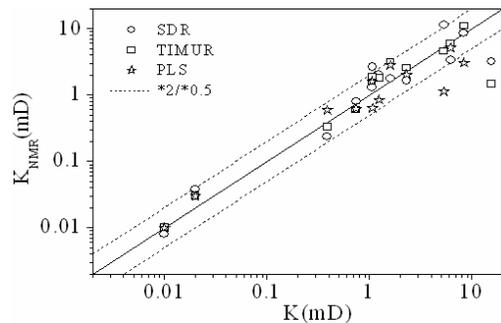
**Figure 3.** Absolute permeability (K) x core NMR-derived permeability ( $K_{NMR}$ ), showing a good agreement between the SDR, Timur-Coates and PLS regression.
