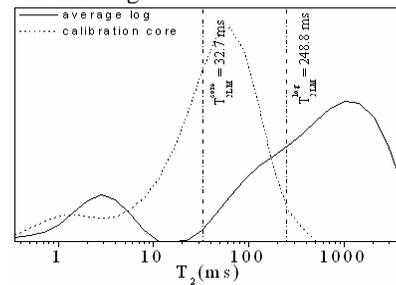
**Figure 5.** Normalized average  $T_2$  log spectra of 15 different depths (4,933.95 to 4,935.02 m) and a 100% brine saturated calibration sample of 1.60mD.
