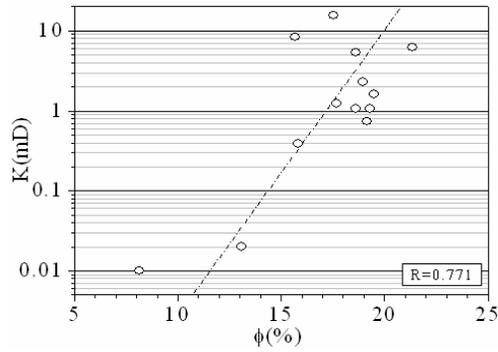
**Figure 1.** Porosity( $\phi$ ) x absolute permeability(K), Klinkenberg corrected.
