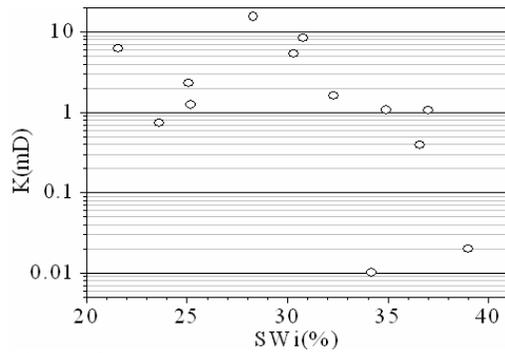
**Figure 2.** Irreducible water saturation (Swi) x absolute permeability (K).
