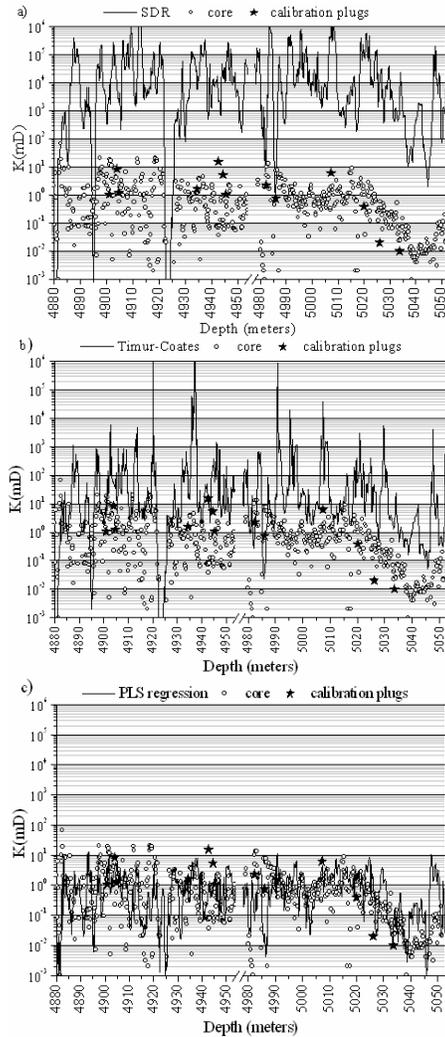
**Figure 4.** Application of calibrated SDR (a), modified Timur-Coates (b) and PLS model (c) to the NMR field log.
