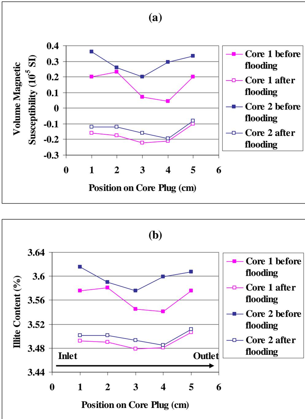
**Figure 2.** (a) Volume magnetic susceptibility determined at various positions (thin slices) on a sandstone core before and after flooding with a seawater brine composition. (b) Corresponding plot of magnetically derived illite content assuming the core plugs comprised a simple two component mixture of quartz and illite. In each diagram the inlet was at position 0 cm and the outlet at position 7.5 cm. The throughput brine volume for Core 1 was 1140 ml and for Core 2 was 798 ml.
