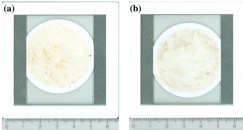
**Figure 4.** Image of fines collected on filter papers (a) at the inlet and (b) outlet of a filter cartridge at the manifold of a water injection pipeline at a North African clastic reservoir.
