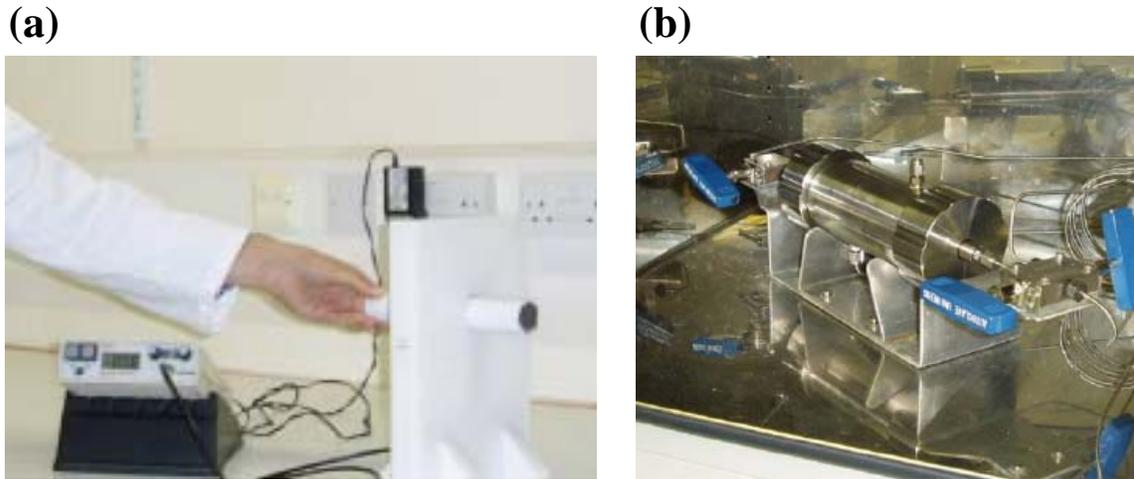
**Figure 1.** (a) Sensor (Bartington MS2C) for measuring low field magnetic susceptibility at points along a core plug before and after core flooding experiments. (b) The flow cell for the flooding experiments.
