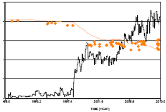
Figure 9. History match of liquid rate and average static bottom hole pressure (all wells) for the flank area B in Case 2.
