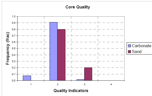
Figure 3. Frequency of quality of core material from 108 individual coring jobs (1 good -4 poor).
