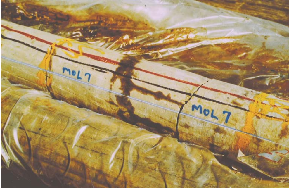
Figure 3 Core Marked with a Master Orientation Line
