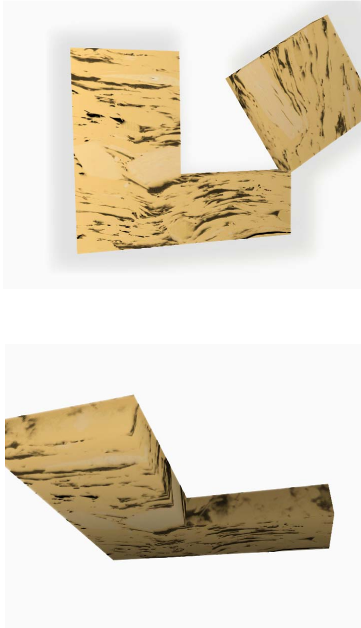
Figure 4. 3D view of the image series shown in Figure 3. The FIB/SEM run consisted of 130 images, with 10 nm slice thickness.
