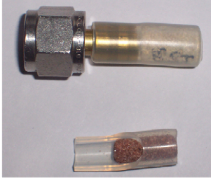
Figure 2 - example of miniplug with the silicone tube
