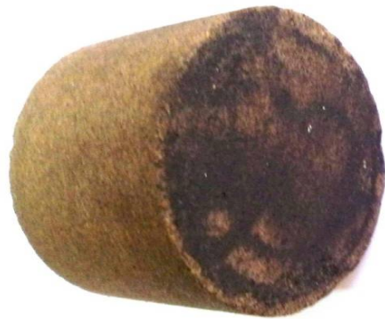
Figure 3- Asphaltene Cake on Injection Side
