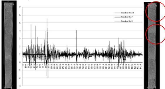
Figure 4: The above figure gives the results of forklift transport (test 3) with non stabilized core and CT-scans before (left) and after test (right). Structural damaged are circled in red. Hard layer foam inserts were used (Test#161).
