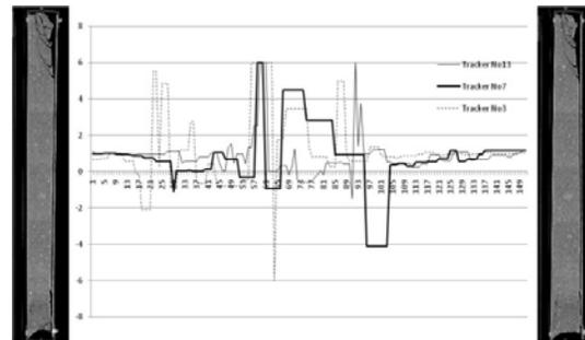
Figure 3: The above figure gives the results of angular shock (test 2) with foam stabilized core and CT-scans before (left) and after test (right). No structural damaged were recorded after test. Hard layer foam inserts were used (Test#82).
