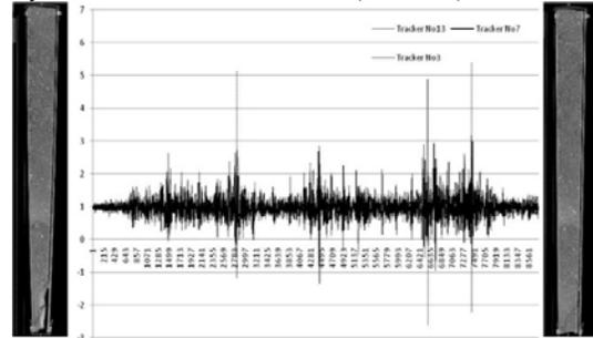
Figure 5: The above figure gives the results of forklift transport (test 3) with foam stabilized core and CT-scans before (left) and after test (right). No structural damaged were recorded after test. Hard layer foam inserts were used (Test#162).
