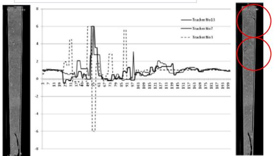
Figure 2: The above figure gives the results of angular shock (test 2) with non stabilized core and CT-scans before (left) and after test (right). Structural damaged are circled in red. Hard layer foam inserts were used (Test#81).
