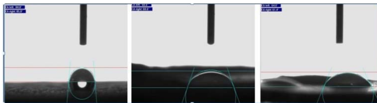
Figure5. Visual illustration of Contact Angle of treated Calcite surface with Stearic Acid (0.01 M) aged for 2 days in different concentrations of Nonionic Surfactant solutions.
