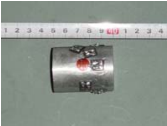
Figure 4. strain gauges are glued on the aluminum sample.
