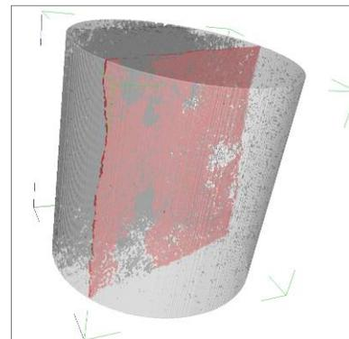
Figure 4. A fractured sample of the Middle Bunter formation: CT image of a cylindrical detail (diameter and length 5 mm).
