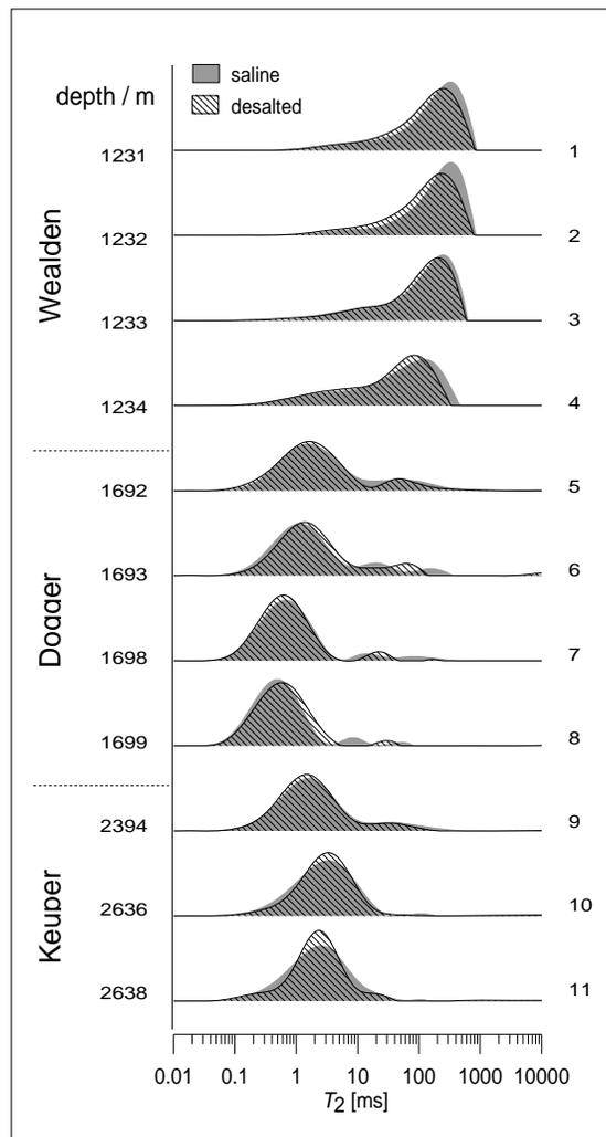
Figure 1.  $T_2$  relaxation time distributions of sidewall cores from the formation Wealden, Dogger and Keuper before and after desalination.
