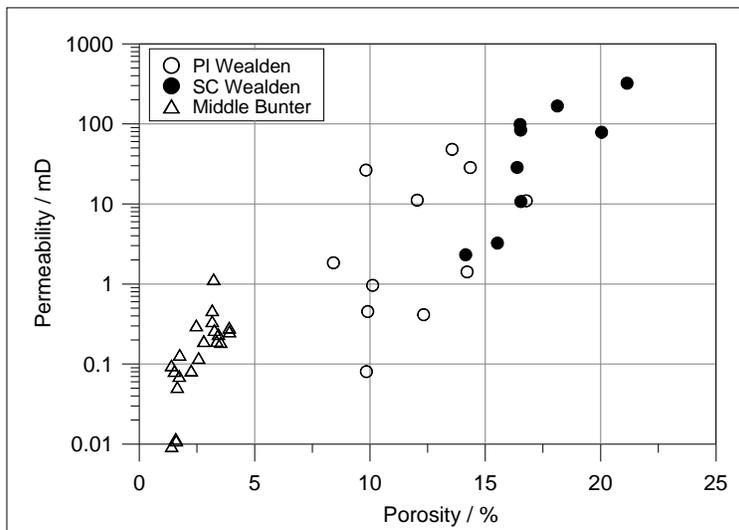
Figure 3. Permeability-Porosity plot for plugs (PI) and sidewall cores (SC) from the Wealden and plugs from the Middle Bunter formation (permeability calculated from NMR measurements, porosity measured by buoyancy method).
