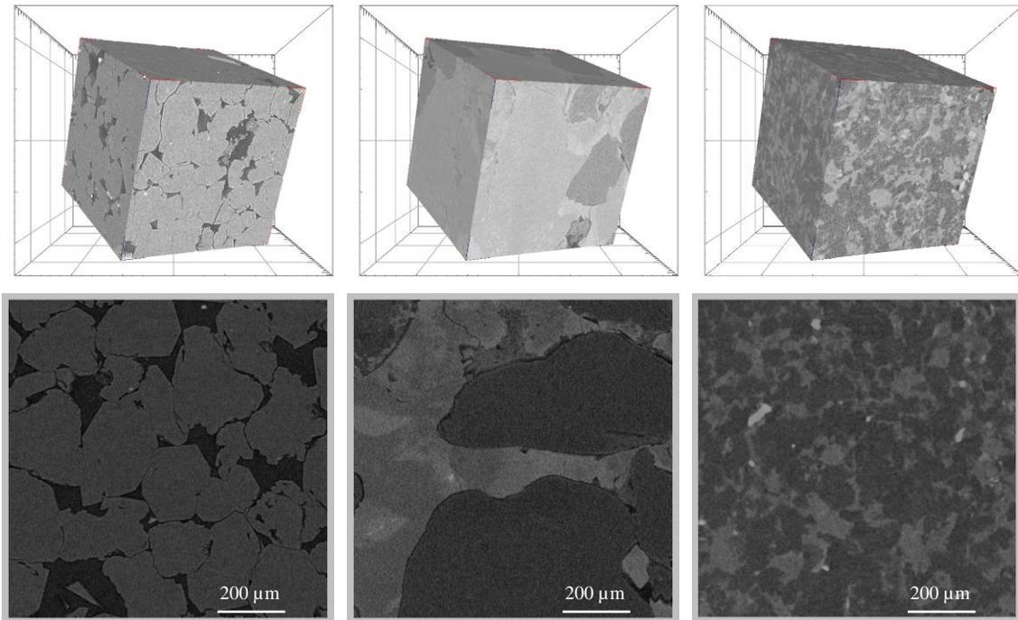
Figure 2. Micro-CT images of a Wealden, Dogger and Middle Bunter Sandstone sample (from left to right). The pore space (colored black) is clearly evident only in the Wealden sample. The achieved Voxel-Resolution is about 1 μm, the volume of the visualized ROI is about 1 mm<sup>3</sup>.
