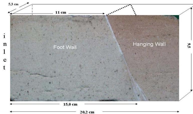
Figure 2. The block sample with dimensions
