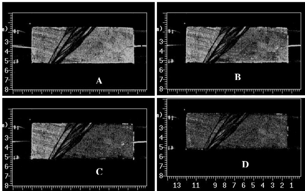
Figure 4: Waterflood in core with deformation band (low rate). Oil (appearing bright) displaced by  $D_2O$  from right. A)  $S_w=29\%$  B)  $S_w=50\%$ , C)  $S_w=60\%$ , D)  $S_w=66\%$ .
