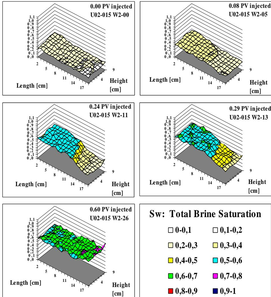
Figure 2. Saturation development when waterflooding the sandstone block. The water halts and forms a front before crossing the deformation band (middle left image).
