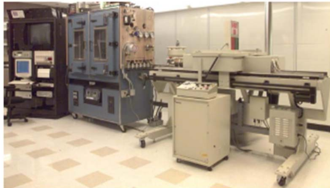
Figure 7. Recirculating relative permeability apparatus with oven and core connected by heat-traced tubing.
