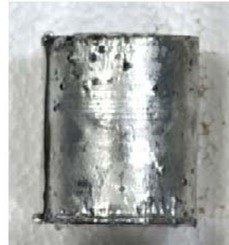
Figure 2. Tin-wrapped unconsolidated core plug showing holes from “tin pest” after long-term cold storage.
