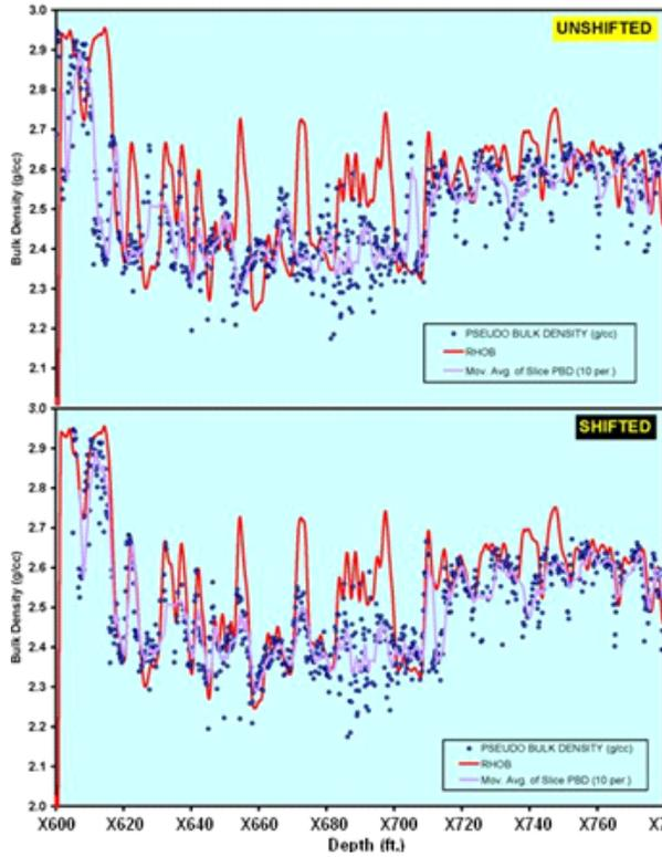
Figure 7. Carbonate Core depth shift using bulk density log and pseudo-bulk density (PBD).
