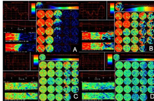
Figure 9. Two-phase displacement in composite core. After partial oil injection (A) at  $S_{wir}$  (B) after 1 PV waterflood (C) after 20 PV waterflood (D).
