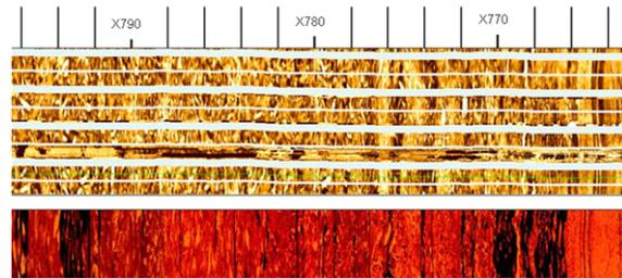
Figure 6. FMI (top slices) and unrolled CT image for carbonate core.
