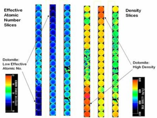
Figure 8. Computed results from dual Energy CT scans 140 kVp and 80 kVp.
