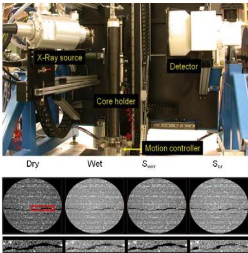
Figure 10. Two-phase fracture flow in micro-CT system.
