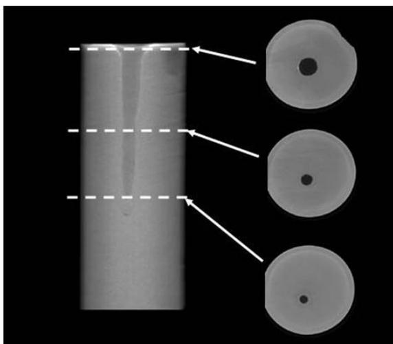
Figure 12. CT inspection of perforation shot penetration.
