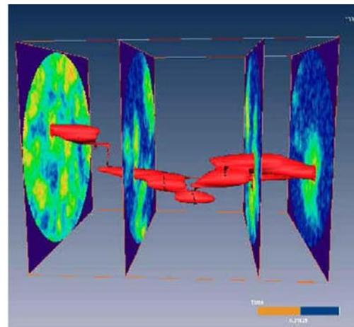
Figure 11. CT observed wormhole development due to acid.
