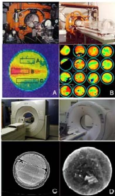
Figure 3. CT Generation machines. 2<sup>nd</sup> Generation Delta-Scan 100 (A) Core flooding 1984 (B) Reservoir characterization 2000 (C) Fourth Generation Picker axial slice (D) Single slice from Helical Scan Acquilon.
