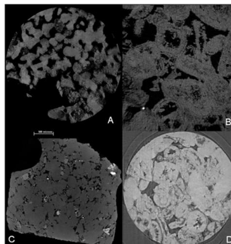
Figure 13. Micro-CT images. Recent sediment (A) Jurassic carbonate (B) Permian sandstone (C) Synchrotron image, Jurassic carbonate (D).
