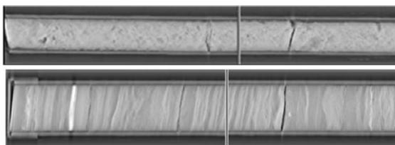
Figure 5. Pilot or Scout images for 2 5/8 in. carbonate core and 4 in. sandstone core.
