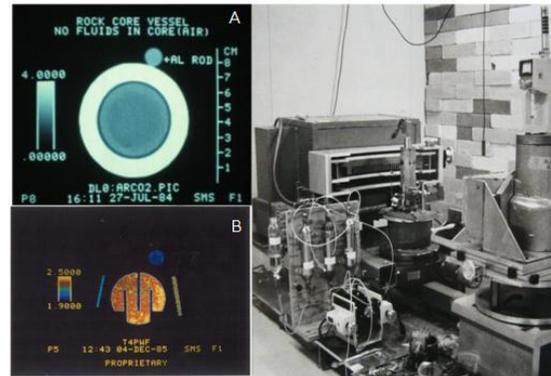
Figure 2. Early material inspection gamma-scan system used for core flow visualization (A) (Withjack, 1984) core flood (B) serpentine flow study.
