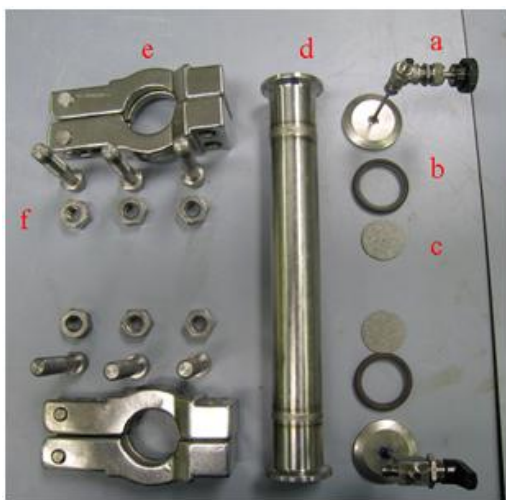
Figure 1: Sand Pack Assembly, including a) End Pieces with Valves; b) Viton O-ring; c) Stainless Steel Frit; d) Pipe; e) Clamp; f) Nuts and Bolts
