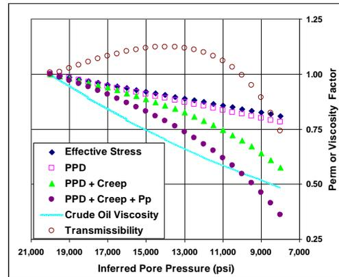
Figure 6B: Perm Factor versus Pore Pressure
