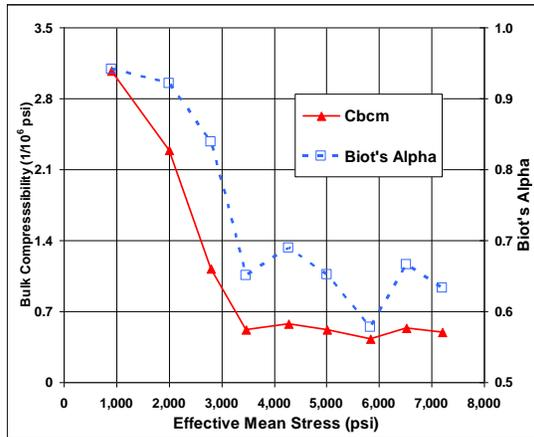
Figure 3A: Bulk compressibility and Biot's Alpha versus mean stress
