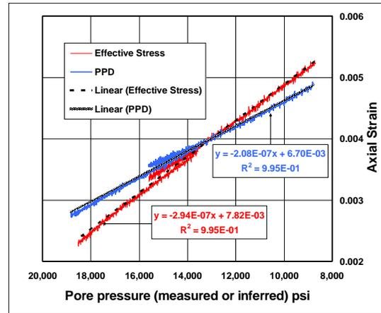
Figure 3B: Calculation of Biot's Alpha from slopes of axial strain versus pore pressure
