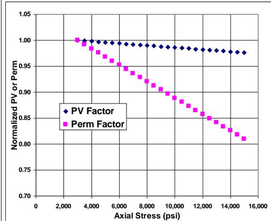
Figure 2: Pore Volume and Perm Factor versus axial Stress
