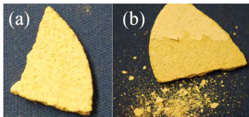
Figure 5: Carbonate substrates treated by 0.5%wt anionic chemical Z diluted in DIW at different temperatures of: a) 130°C and b) 160 and 190°C. A deposited layer of chemical is evident on the treated rocks at two higher temperatures (b).
