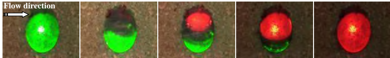
Figure 4: Vug filling during primary drainage (brine in green and oil in red).
