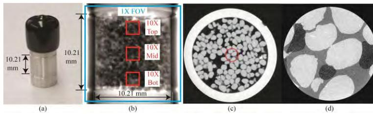
Figure 1: Picture of the partially saturated sand specimen (a), radiography of partially saturated sand specimen showing 1X and 10X magnification FOV size and location (b), tomography slice of partially saturated sand specimen at 1X magnification (c), and tomography slice of partially saturated sand specimen at 10X magnification (d)
