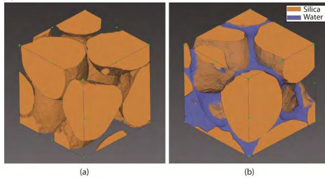
Figure 2: Three dimensional visualization ( $1\text{mm}^3$ ) of dry (a) and partially saturated (b) sand specimen at 10X magnification
