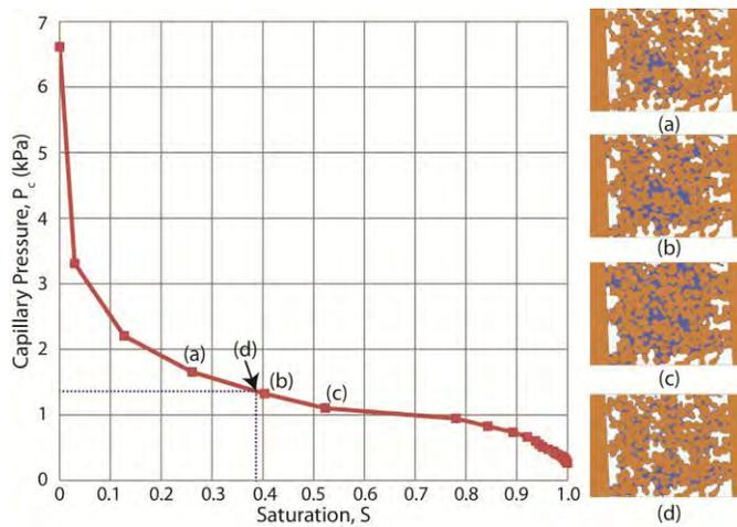
Figure 3: Simulated capillary pressure saturation curve of drainage and example two phase distributions from simulation (a, b, c) and experiment (d)
