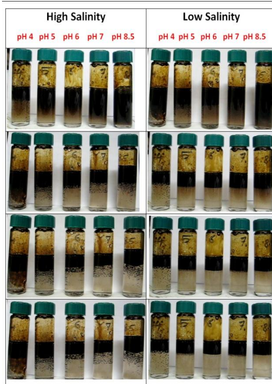
Figure 8. Snapshots taken at same time to show the difference in between the settling rates of the emulsions formed for HS and LS brine at t = 20,50,80,100 secs.
