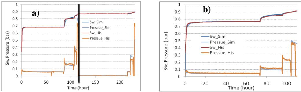
Figure 5: a) Tertiary and b) secondary LSF core floods with the history-matched data
