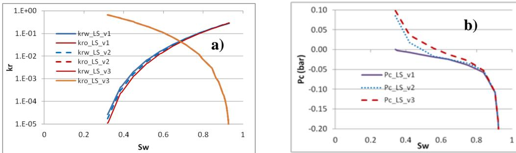
Figure 7: a) HS and LS relative permeability curves and b) Pc curves that history match the data shown in Figure 5.
