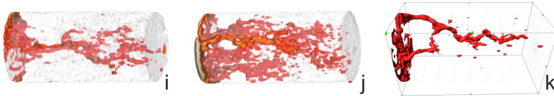
Figure 7: CT difference images of dissolution patterns in Euville limestone that have been formed after 3 (i) and 6 (j) retarded acid treatments and during injection of CO 2 -saturated brine (k). Note that the CT contrast of i and j is strongly enhanced compared to the contrast of image k. The initial rock-fluid system is displayed as a semi-transparent background.
