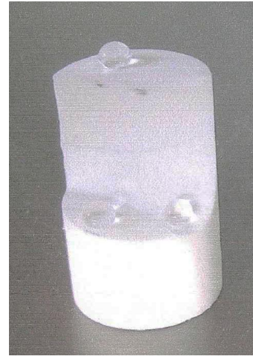
Figure 4: Porous borosilicate sample (diameter: 2 cm, height: 3 cm) with water drops on hydrophobic inner surface.
