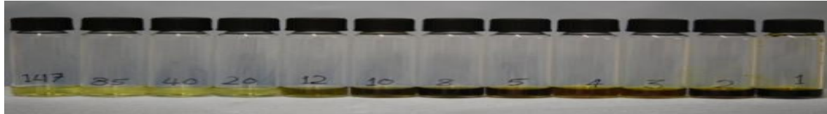
Figure 6: Right to Left: shows the effluent samples obtained by injecting the core sample with methanol after it was flooded with the magnetic tracer. The light muddy color of the effluent samples (far left) indicates that the magnetic tracer has not been flushed out of the core sample fully and is continuously being produced at smaller concentrations. Dark colored samples (far right) indicate higher concentration of the magnetic tracer in the solution at the start of methanol injection.
