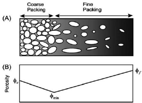
**Figure 1** Ideal packing model. (a) for a binary mixture of grains in which either fine grains fill the space between coarse grains or coarse grains are dispersed among fine sediments (b) porosity as a function of fine and coarse grains. Minimum porosity occurs when the amount of fine grains is equal to the porosity of coarse grains [9].
