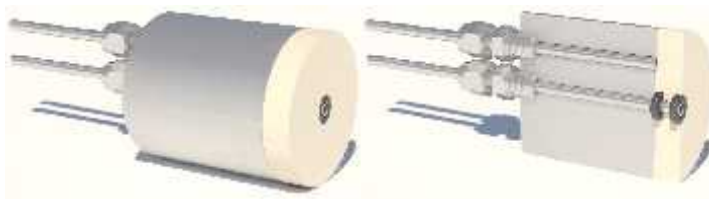
Figure 2. The modified porous plate is attached to the end of a steel platen which houses the two flow lines. Rubber o-rings form a seal in-between the porous plate and the central steel flow line preventing the bypassing of fluids.
