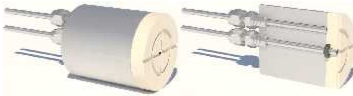
Figure 4. The porous plate could be modified further by the inclusion of flow distribution channels, allowing injection water to access a greater fraction of the core-plug cross section.
