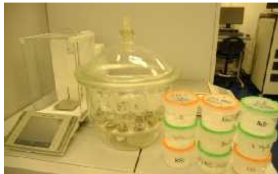
Figure 2. Adsorption isotherm measurement setup.
