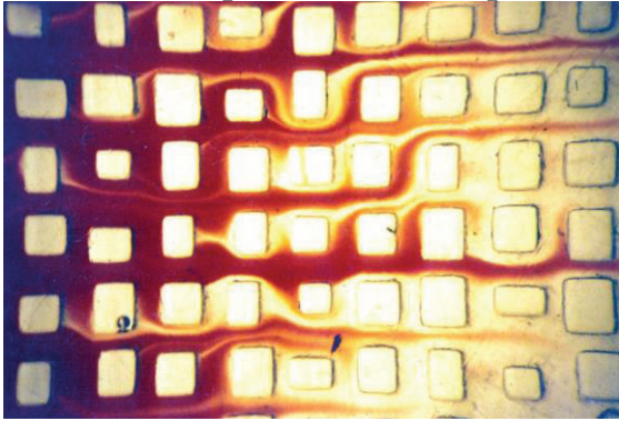
Figure 1- Tracer flow experiment in a micromodel. The tracer in red is injected at a constant flux on the left
