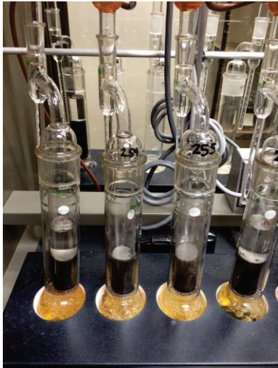
Fig. 5A - Dean Stark extraction apparatus showing orange discoloration of toluene in boiling flask. The discoloration resulted from hydrocarbons released after crushing a core plug that had already been subjected to RCA Dean Stark cleaning
