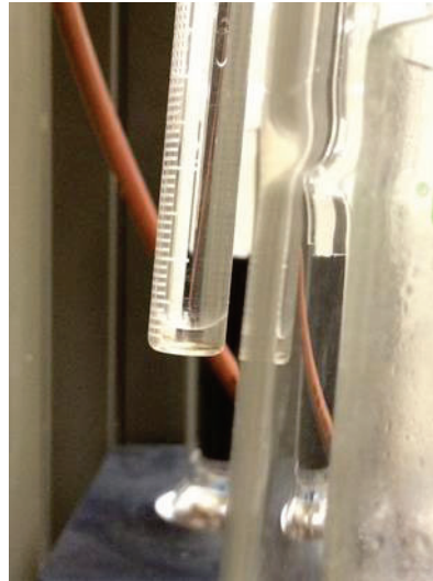
Fig. 5B - Water level in the calibrated receiver of the Dean Stark extraction apparatus. This additional water was extracted from the sample after crushing a core plug that had already been subjected to 'complete' RCA Dean Stark cleaning
