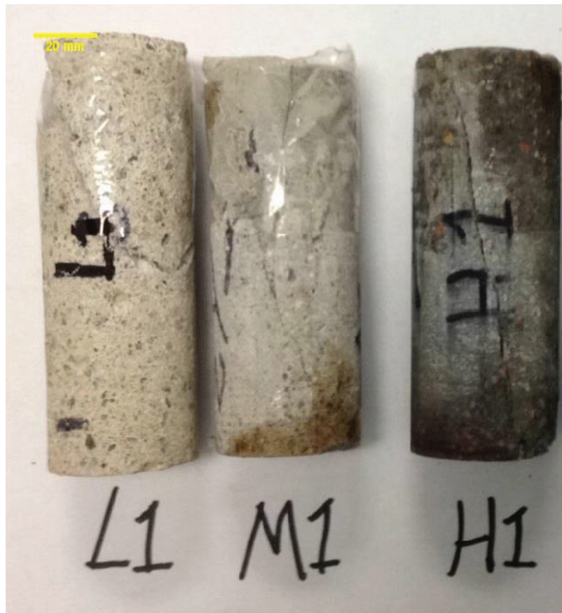
Figure 11. Post failure illustration for low, medium and high strength cores under confining pressure of 2 MPa.
