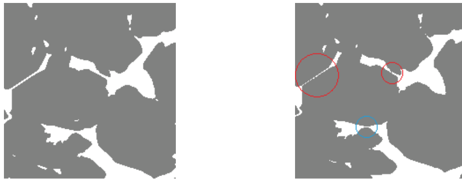
Figure 2 Cut-out from the segmented image of Berea sandstone before (left) and after (right) numerical compression (1.43 GPa). The pore diameter in the blue region is visibly decreased while even the connectivity of the pores is reduced in the two red regions.
