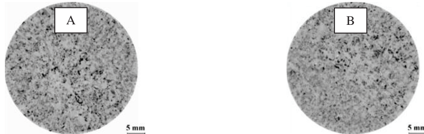
Figure 3: Typical 2D micro-CT cross-sections obtained from conventional sample IL4 (A) and from sidewall sample IL14 (B)
