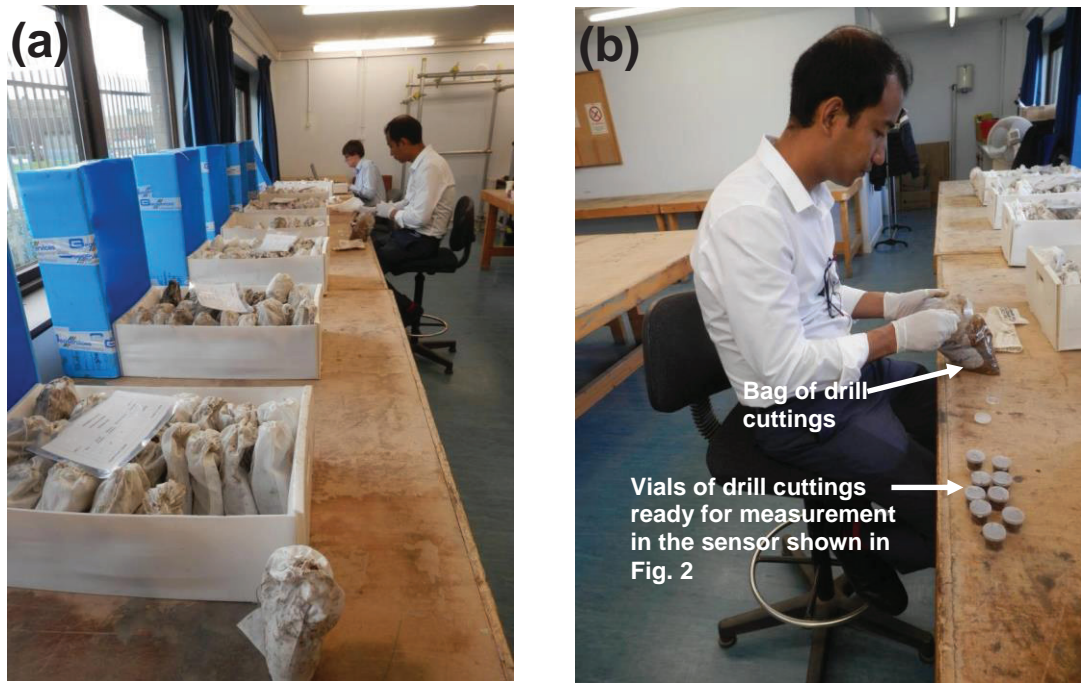
Figure 1. (a) Bags of drill cuttings arranged in order of their depth in the well. (b) Samples of drill cuttings being put into the vials for measurement.
