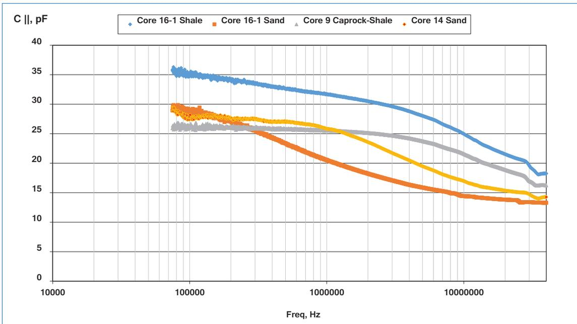
Figure 9: Capacitance comparison for shale vs. sand
