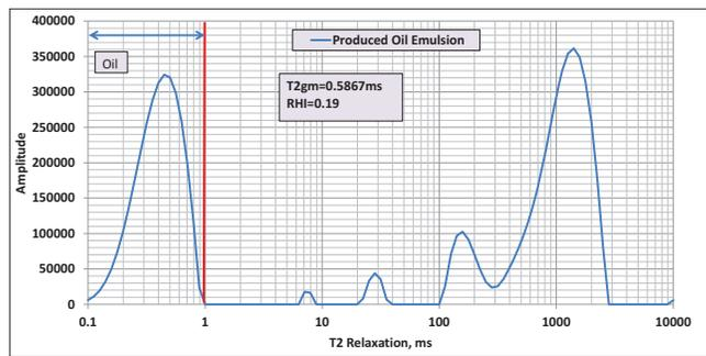
**Figure 2:** T<sub>2</sub> relaxation distribution of produced bitumen emulsion
