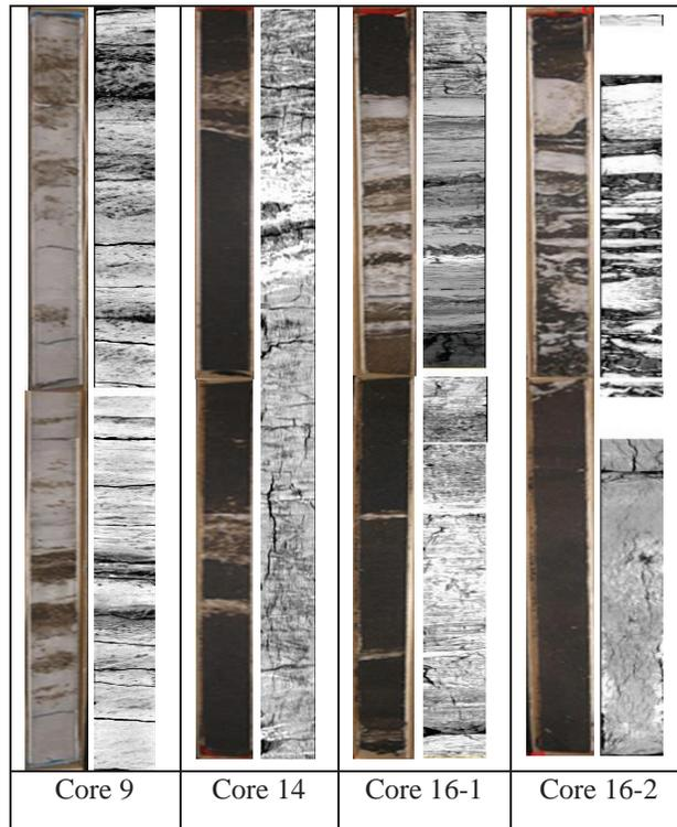
**Figure 1:** Core photos and corresponding CT image sequences
