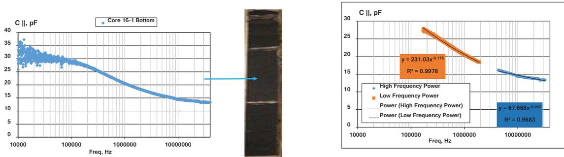
Figure 7: EM sweep and power fit from an oil sand sample
