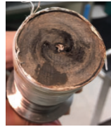
Figure 5: Spiral with gasket end-piece after exposure to live crude oil at high pressure and temperature. Incompatible material was used in this test.
