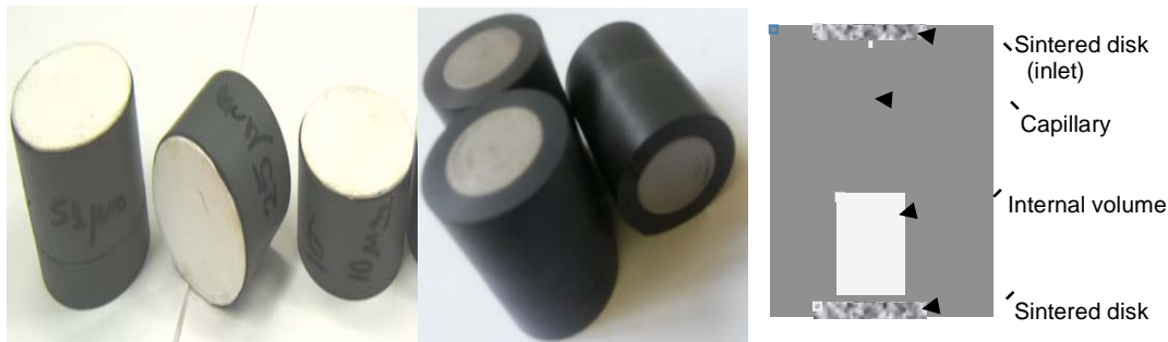
Figure 1. Photos and schematic of the reference plugs of 38mm diameter; left: first set; centre: second set; and right: schematic of the second set.
