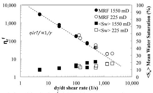
Figure 8: The foam relative viscosity  $\eta_r^f$  (circles) and the mean water saturation  $\langle S_w \rangle$  (squares) vs. the shear rate  $\dot{\gamma}$  computed from eq. (2) in Clashach sandstone at 30°C and a pore pressure of 10 bar. The full symbols represent data for a 1550 mD sandstone with a porosity about 20%. The empty symbols for 225 mD with a porosity about 12%. The dotted line corresponds to the equation  $\eta_r^f = 16000/\dot{\gamma}$ .
