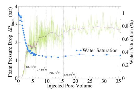
Figure 6: Dense supercritical  $CO_2$ -foam generation in a 820 mD Clashach sandstone. The line in dark purple is a running average of 200 points of the raw pressure drop measurement represented here in light green. The full circles represent the mean water saturation along the core. Data are plotted against the total injected pore volume and thus not linear in time as the total flow rate was increased from 10 up to 300 cm<sup>3</sup>/h.
