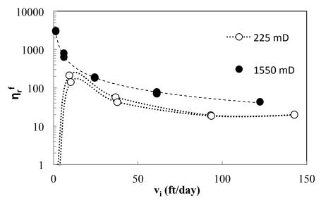
Figure 4: Foam relative viscosity in a small core of Clashach sandstone plotted against the interstitial velocity. Full circles correspond to the date obtain with a core of 1550 mD water permeability and 20.2% of porosity. Empty circles are the data for 225 mD and 12.1% porosity. Points are obtained with both increasing and decreasing velocities (duplicate points).
