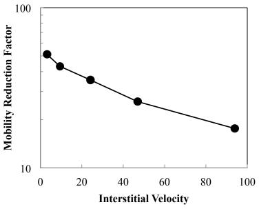
Figure 7: Mobility Reduction Factor evaluated from the performance ratio between foam and gas/water coinjection MRF =  $\Delta P_{\text{foam}}/\Delta P_{\text{water-gas}}$ . The  $\Delta P_{\text{water-gas}}$  is extracted from the linear regression of raw data (Figure 5).
