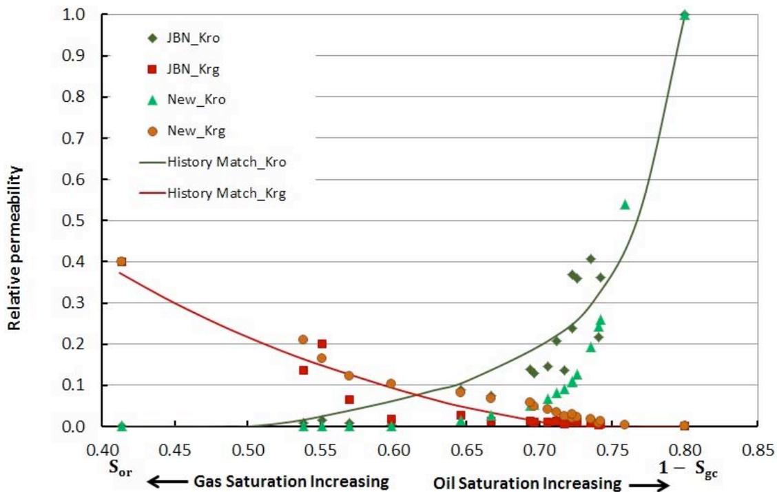
Figure 2 Gas-oil relative permeability results
