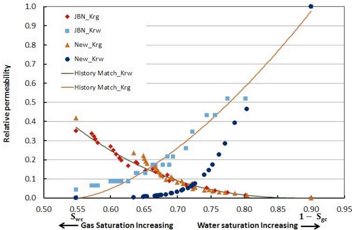
Figure 3 Gas-water relative permeability results
