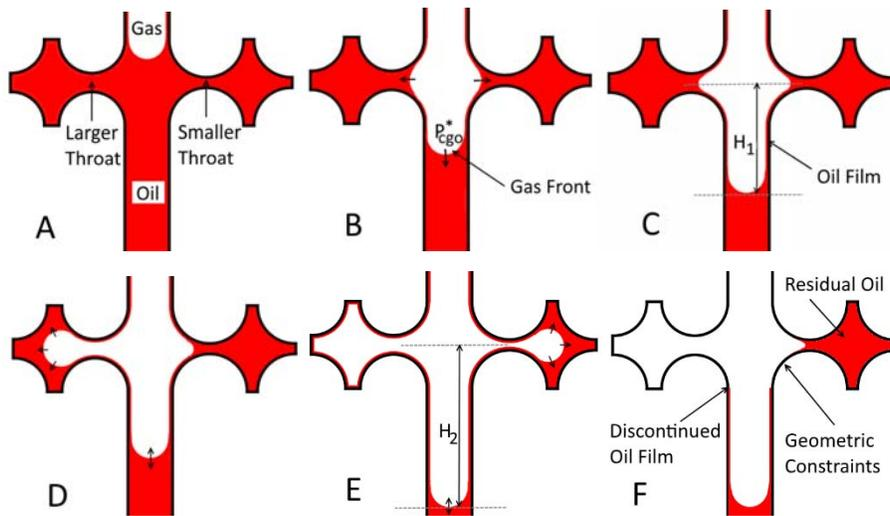
Fig. 1: Oil drainage behind the gas front through film flow in capillary corners
