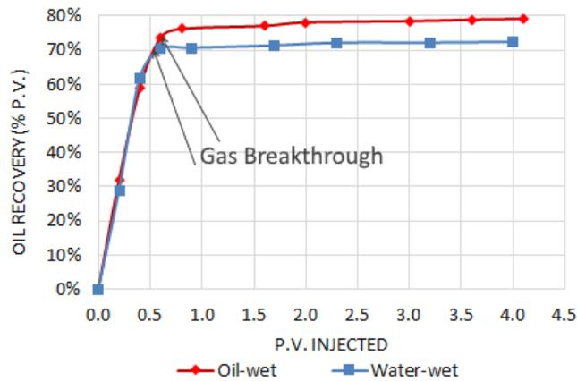
Fig. 4: Oil recovery curve in both states of wettability vs. pore volume of injected gas
