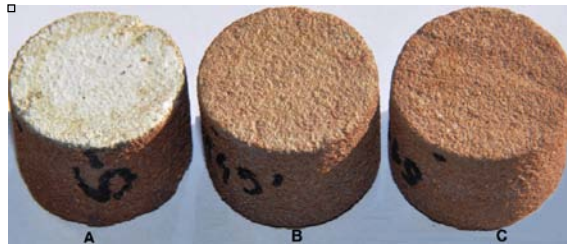
Figure 2. The Rotliegend Sandstone cores after the injection of A-cross-linked polymer, B-linear polymer, C-slick water.
