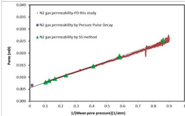
**Figure 4.** Sample S4: Gas permeability by 1) unsteady-state pressure decay (draw-down) using (N2) Nitrogen; 2) pressure pulse decay measurements using N2 gas; 3) gas permeability measured by steady-state method.
