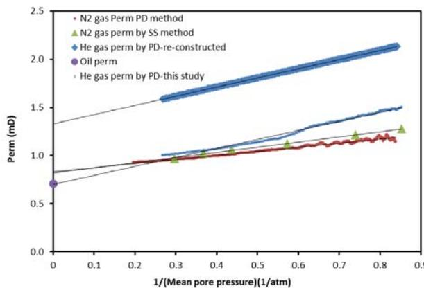
**Figure 2.** Sample S2: Klinkenberg permeability measured by 1) unsteady-state pressure decay (drawdown) using Nitrogen; 2)Klinkenberg permeability measured by steady-state method using N2 gas (green triangle); 3)permeability of lab oil (dot). 4)unsteady-state pressure decay for Helium calculated by Jones method; 5) unsteady-state pressure decay (draw-down) using Helium calculated by Brace’s method.
