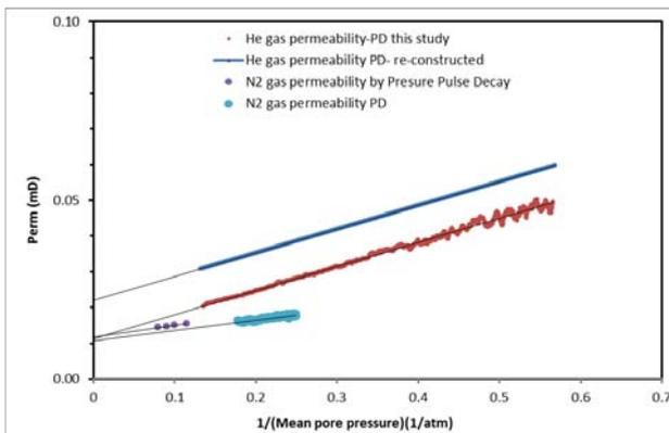
**Figure 3.** Sample S3: Klinkenberg permeability by 1) unsteady-state pressure decay (draw-down) using Helium; 2) unsteady-state pressure decay (draw-down) using (N2) Nitrogen; 3)Klinkenberg permeability by four pressure pulse decay measurements using N2 gas; 4)unsteady- state pressure decay for Helium calculated by Jones method.
