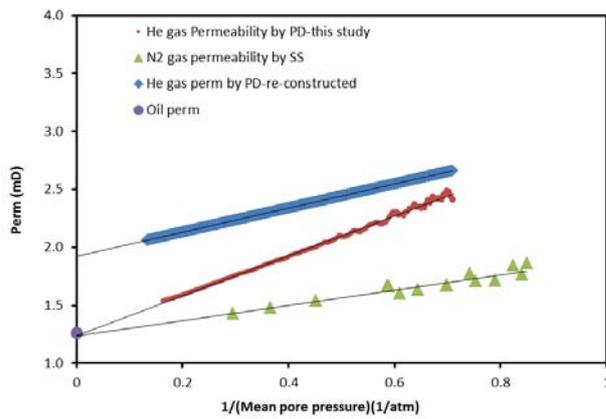
**Figure 1.** Sample S1: Klinkenberg permeability measured by 1) unsteady-state pressure decay (draw-down) using Helium; 2)Klinkenberg permeability measured by steady-state method using N2 gas (green triangle); 3)permeability of lab oil (purple dot).
