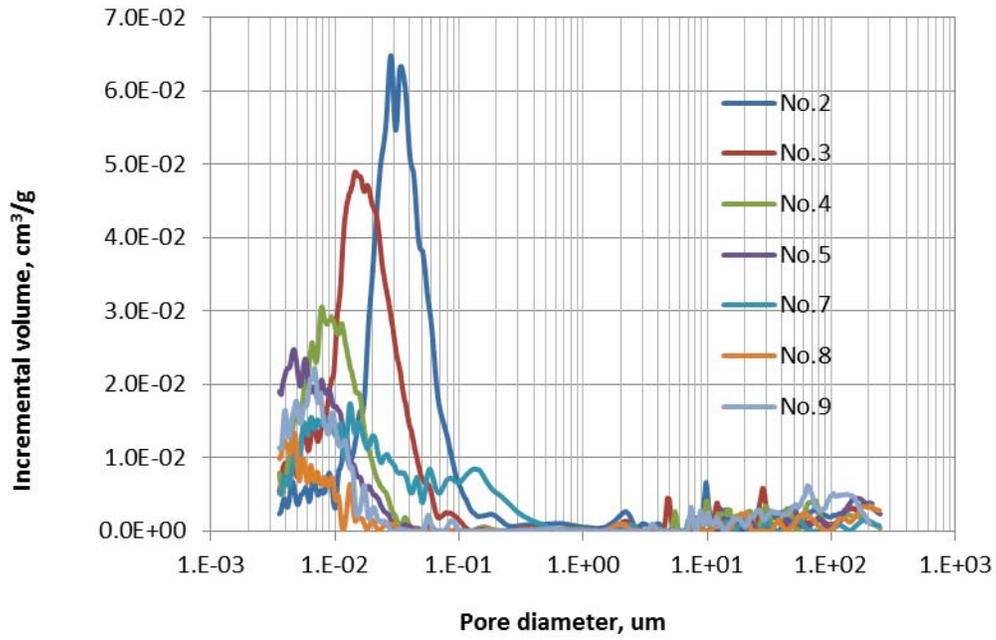
Fig.1 Pore throat distribution by MICP.
