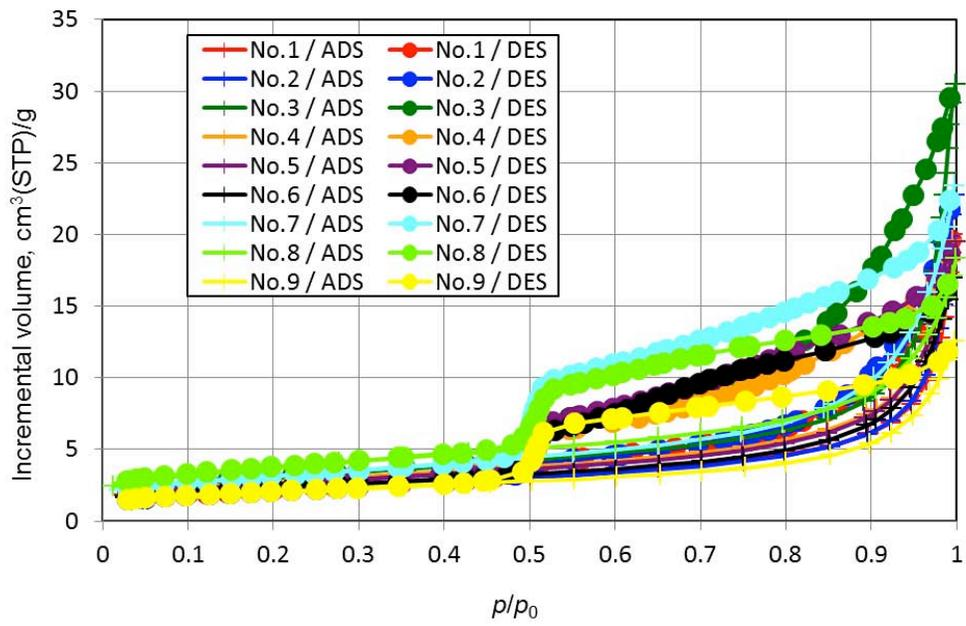
Fig.3 Adsorption and desorption isotherm.
