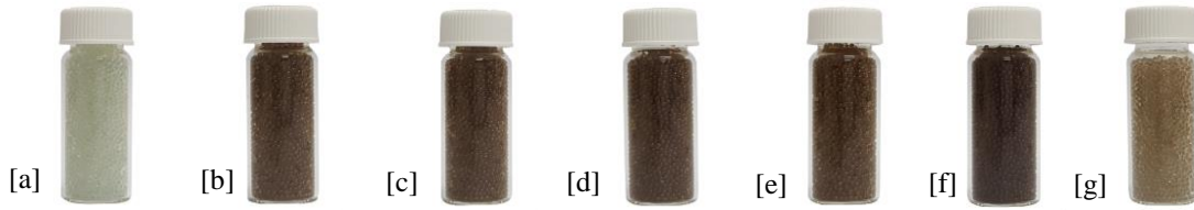
Figure 2. Reference 20 cc borosilicate beadpack [a] and beadpacks aged 14 days in different natural and synthetic oils (dried): [b] oil 0.a; [c] oil 1.b; [d] oil 2.c; [e] oil 3.d; [f] oil 4.e; [g] crude oil.
