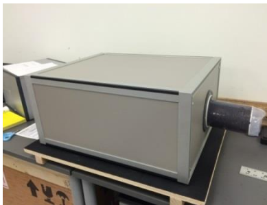
Fig. 3: Illustration of a whole core in Teflon shrink-wrap in the spectrometer probe. The large gray box encloses the magnet and rf -coil. A separate box on the left contains the control console and the rf amplifier.
