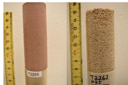
Figure 3: Sample number 1 (left) and sample number 2 (right) before triaxial testing.
