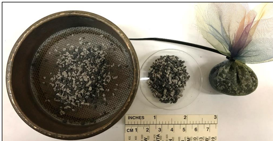
Fig. 2 Cutting samples were sieved, then collected in PTFE filter mesh bag, ready for the saturation process.
