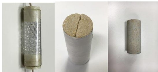
Figure 1. (left) sample A: glass beads pack (37 % in porosity); (middle) sample B: fractured sandstone (18.44 % in porosity); (right) sample C: sandstone (16.28 % in porosity).
