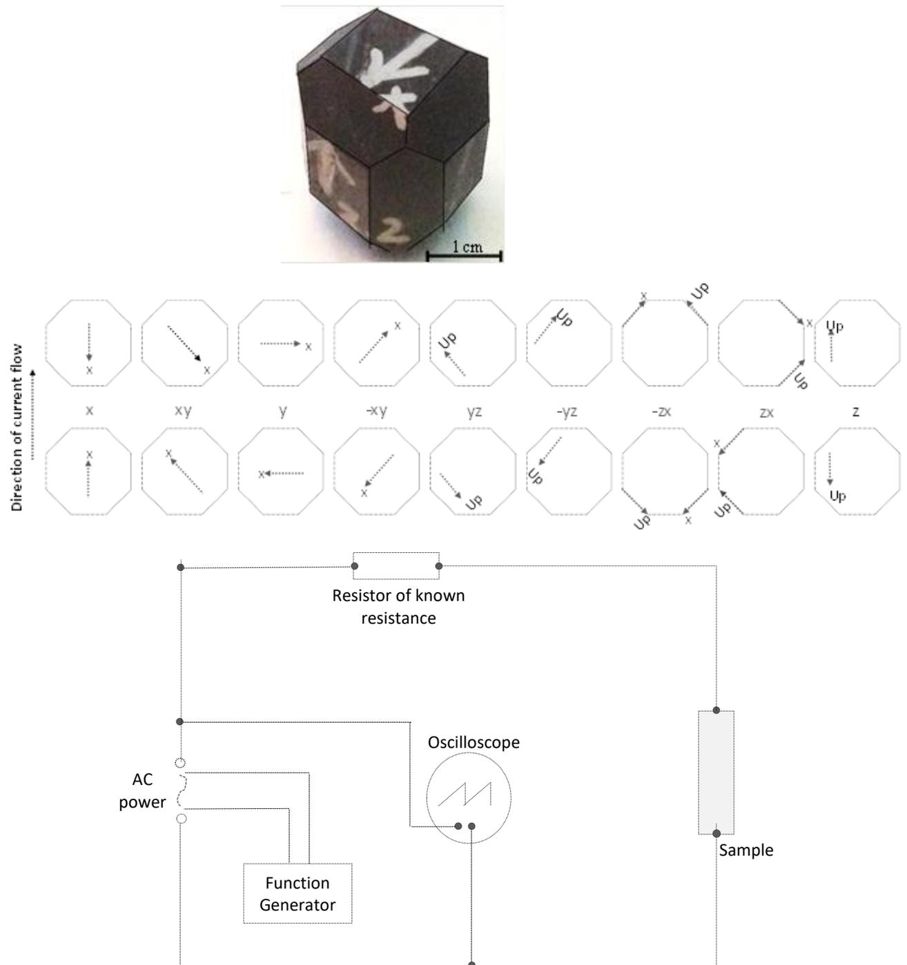
**Figure 1. Top:** One of the 18 sided samples that allow resistance measurements to be made in 9 different sample axes. **Middle:** Schematic of the 18 measurement directions along 9 different sample axes. **Bottom:** Schematic of the experimental set-up for resistance measurements.
